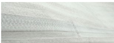
GORE™ Seam Tape intact after 18 months of service.
